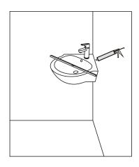
3) Take away the basin, use Ø10mm driller to make four 60mm depth holes following the marks.
