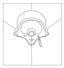
4) Put the expanding plastic into the hole, then fix the bolt with 60mm out of the hole.
