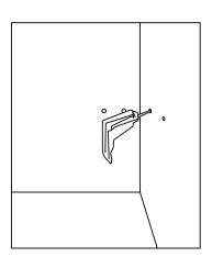
2) Someone holds the bsain on its place ,the other one remove the pedestal away,then put marks on the wall for the installing holes (two).
